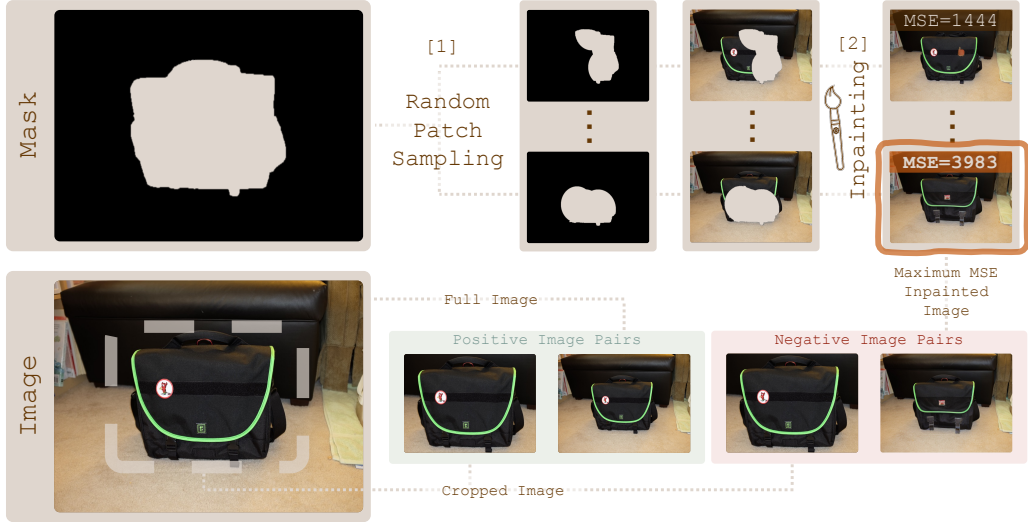
Figure 4: Creating identity-sensitive \{image_{ref}, image_{tgt}\} pairs. Starting with an image and a mask of a subject (e.g., a bag), we randomly keep 5 patches within the masked area ([1]) and use them to create 5 inpainted versions ([2]). The version with the highest MSE between the altered and original areas (e.g., bottom image, MSE = 3983) is paired with the unmodified crop to form a negative pair , while the original image and the same crop create a positive pair , with the crop acting as image_{ref} in both cases.
